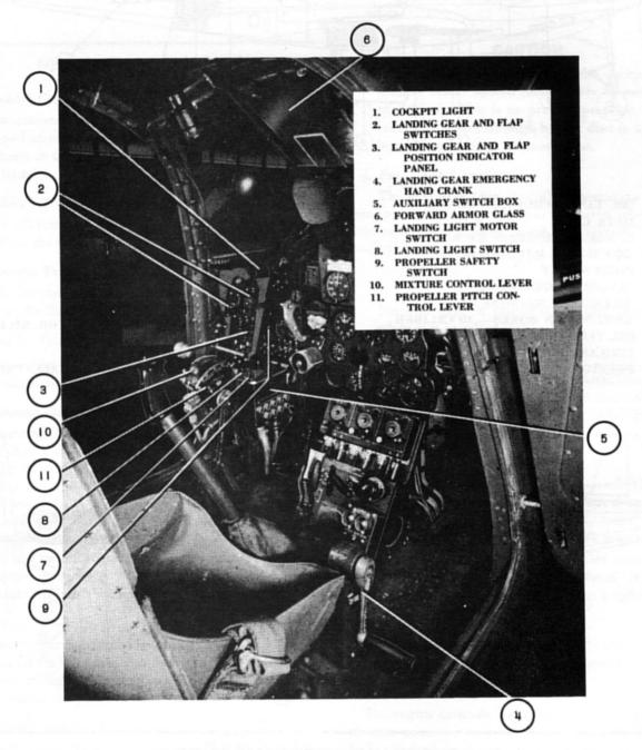
Figure 6—Cockpit, Right Hand Side of Seat
