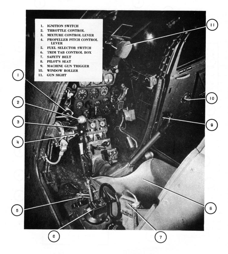
Figure 8-Cockpit, Left Hand Side of Seat
