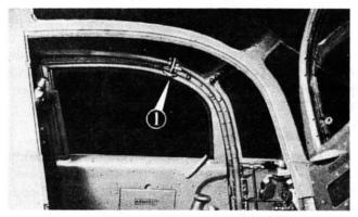
Figure 2-Auxiliary Door Latch
