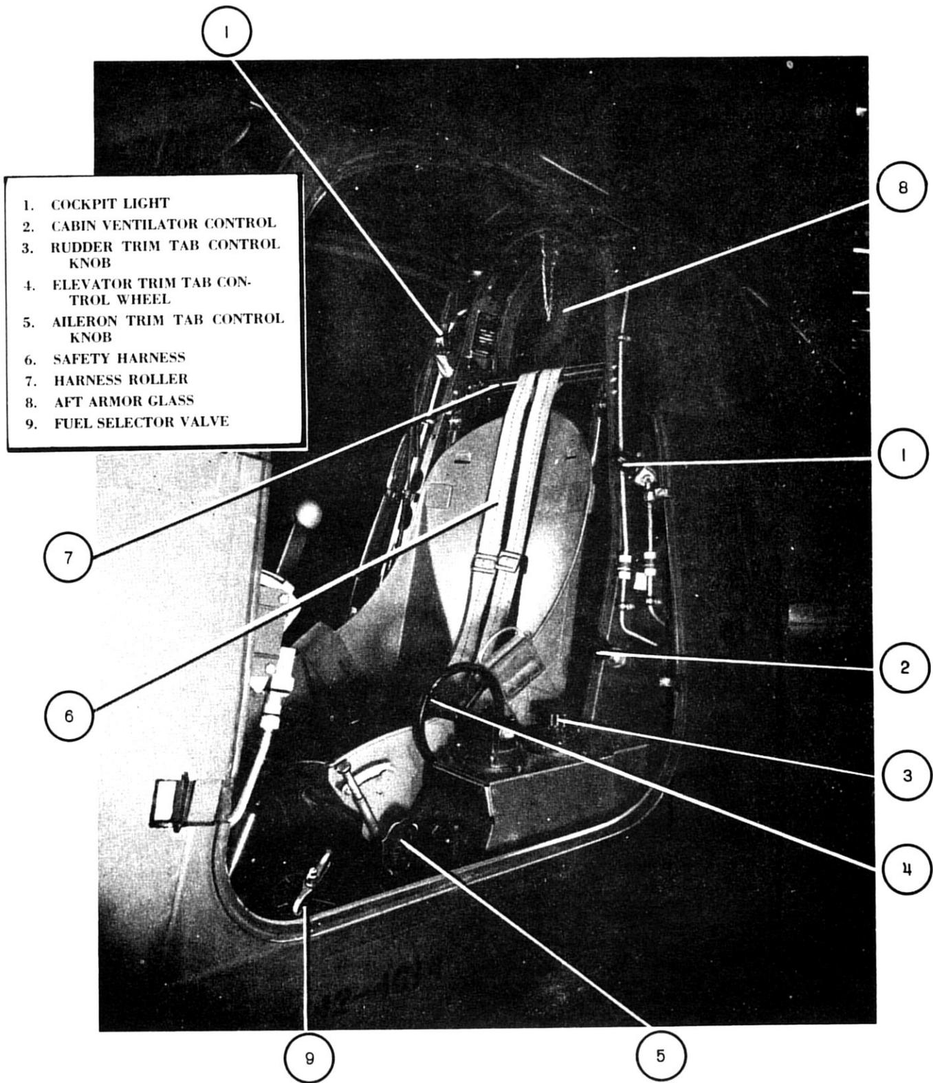
Figure 9—Turnover Beam, Left Hand Side
