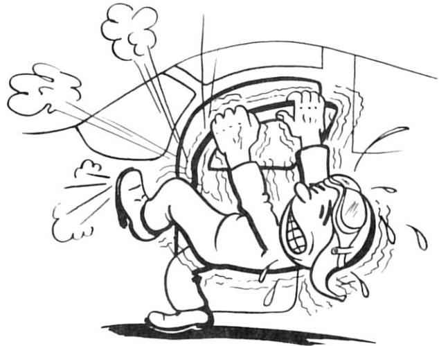
(5) ENTRANCE TO THE COCKPIT is made through the right hand door. The door is opened by pushing in the upper end of the flush handle causing it to hinge out, upon which it can be pulled upward, opening the door.
