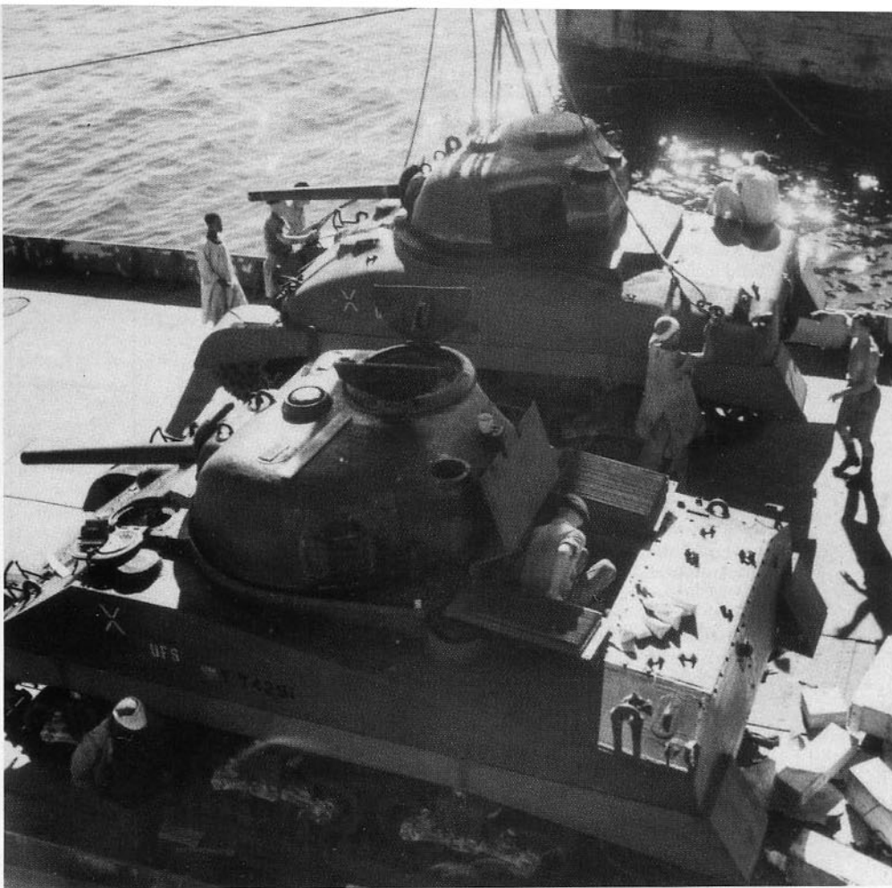
Sherman III (M4A2) T 74291 and Sherman II (M4A1) T 74418 side by side after having been unloaded. These are the first types used by the British and both are painted in US Olive Drab and have their British WD serial numbers painted in Blue Drab on their hull sides. These numbers were applied by American Ordnance from blocks supplied by the British when the vehicles were ordered. The diesel engined Sherman III nearest the camera has had its sealing removed, whereas the Mark II's is still in place, it having just been hoisted from the freighter that carried it to Africa from America. (TWM E16607.)
