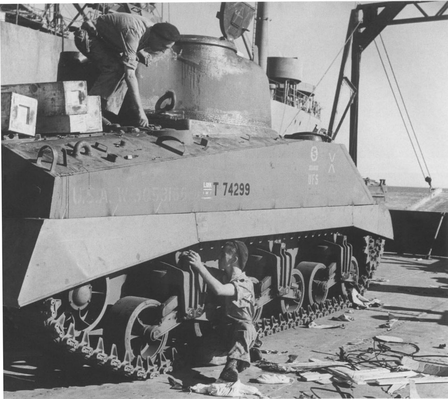
Sherman III T 74299 is prepared by RTR personnel on a 'Z craft' after unloading from the American merchant ship alongside. This photo is interesting in that the Sherman still carries its US serial number (U.S.A. W. 3053166) in very faded Blue Drab and its British serial (T 74299) in newly painted Blue Drab which shows up dark against the faded Olive Drab of the tank. This is one of the vehicles taken from the US armoured divisions to make up the deficit of tanks lost at sea. The temporary link and shipping markings on the hull side are a pinkish red, confirmed by colour footage of Shermans being loaded into ships in the USA. The shiny areas on the turret are where the sealant has been removed. (IWM 16608.)
